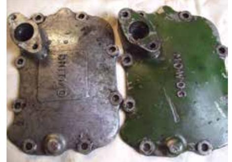
Fig.12. A side cover marked 'Britmo' may identify an earlier 803cc gearbox, but this is not conclusive.
