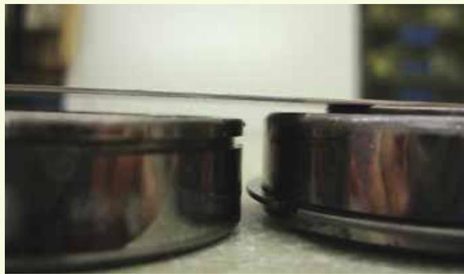
*Fig.6.* The third motion shaft bearing on 1098/1275cc gearboxes (right) is thicker than on the 803/948cc version.
