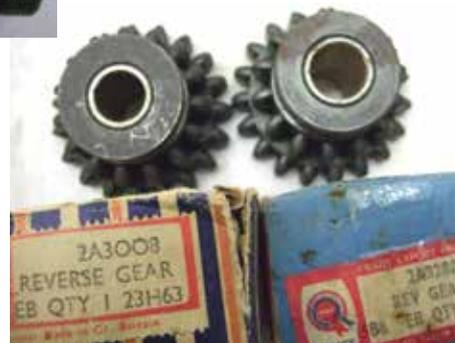
Fig.11. The early Series II reverse gear idler (2A3008), left, runs on a thinner shaft than the later Series II version (2A3280).
