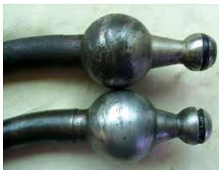
*Fig.8.* The 1098cc gear lever (top) has a longer end section than the 948cc one.
