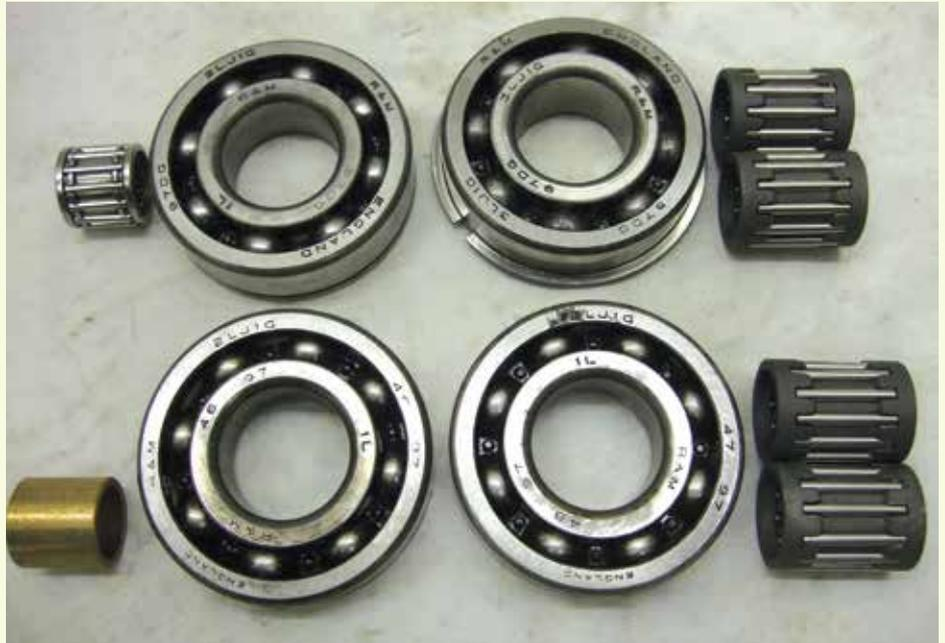
*Fig.7.* Bearings and bushes from the 1098/1275cc box (top row) and 803/948cc version (bottom row). The 803/948cc layshaft bearings, bottom right, are the modern caged type.
