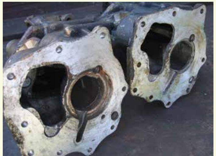
Fig.5. The 1098/1275cc casting (left) has a deeper step in the round hole (counter-bore) than the 803/948cc version (right).
