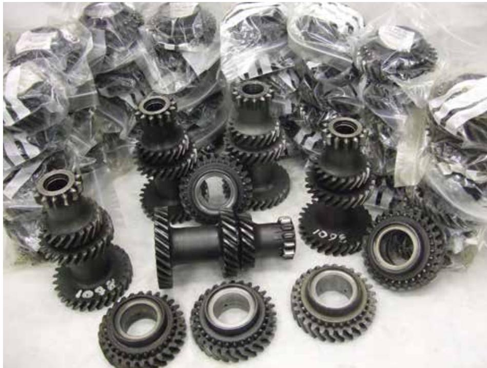
Fig.1. 1098cc laygears and 2nd gears.
