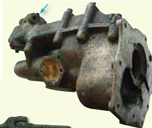
Fig.4. Some late Spridget gearboxes have a screwed port to accommodate the reverse light switch.
